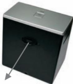
Remove backlight holder by pressing down the handle and pulling it out.
