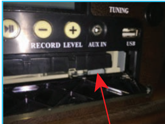
3. Locate the small, silver rectangular button under the CD deck to force open the inner CD door. (shown in the image above.)
