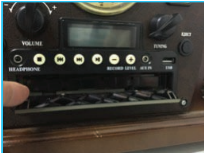
2. Use your finger to pull down the outer CD door. This will allow the outer CD door to open in order to access the inner CD door.
